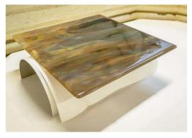
fibre blanket or shelf paper between the mold and the blank will help ensure that the blank will not stick to the mold.
