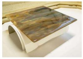
Additionally, using a thin fibre blanket or shelf paper between the mold and the blank will help ensure that the blank will not stick to the mold.
